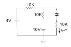
As the 10V source drives an open circuit and the  $10k\Omega$  resistor ends at an open circuit, we can neglect them. Using KVL, we can find the current through the loop using the following equation:
